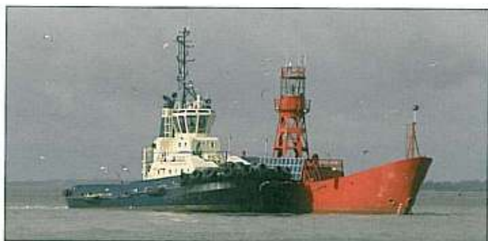
Changing diesel powered light vessels to solar power will dramatically reduce maintenance requirements whilst saving up to 23,000 litres of diesel per vessel per year.
