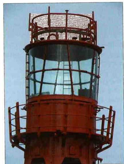
The light vessel's lantern demonstrating space which greatly assists installation and maintenance of the light source.
